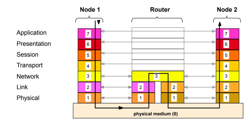
The router routes the frames on the base of their network address.
