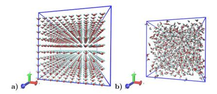
Figure 2: A box of 1000 water molecules (before and after pressure equilibration), generated by moltemplate and visualized by VMD with the topotools plugin. (The VMD console commands used for visualization were: "topo readlammpsdata system.data full", "animate write psf system.psf", "pbc wrap -compound res -all", and "pbc box". See sections 4.3, and C for details.
