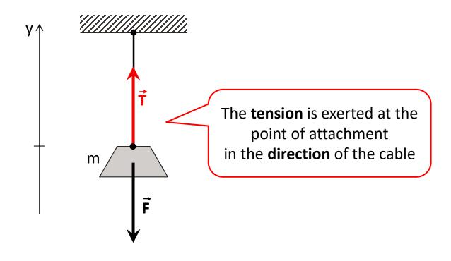
If the object is not moving, then it is in **static equilibrium**. By Newton's First Law (zero net force), the tension in the cable is :  $\overrightarrow{\tau} + \overrightarrow{c} = \overrightarrow{\Delta}$
